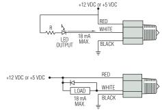
Note: Inductive loads must be diode suppressed.
